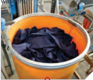
Garments being automatically loaded into continuous batch washer.
