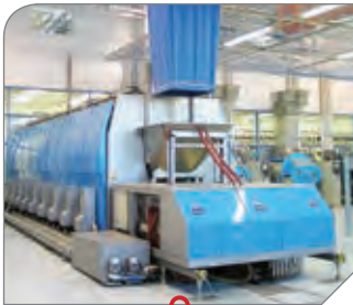
Garments being automatically loaded into continuous batch washer.
