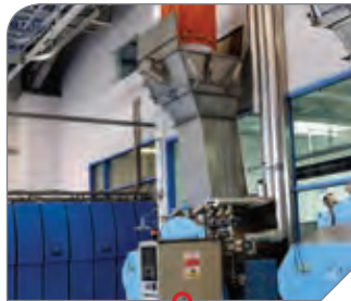
Garments being automatically loaded into continuous batch washer.
