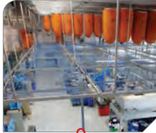
Garments being automatically loaded into continuous batch washer.
