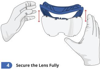
Gradually press along the edges while working your way around the lens.
