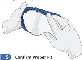
Check that the lens is fully seated in the frame with no gaps. Lightly press around the edges to ensure
