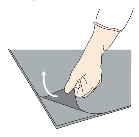
4 Before removing the cover marked 'This Side Up', walk on mat to increase adhesion to floor.
