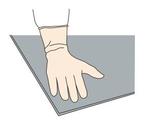
Remove all the packaging including the outer polythene film. From the bottom surface remove the protective layer covering the floor adhesive.
